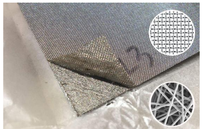
Sintered Metal Fiber Felt With Woven Mesh As Protection Layer
