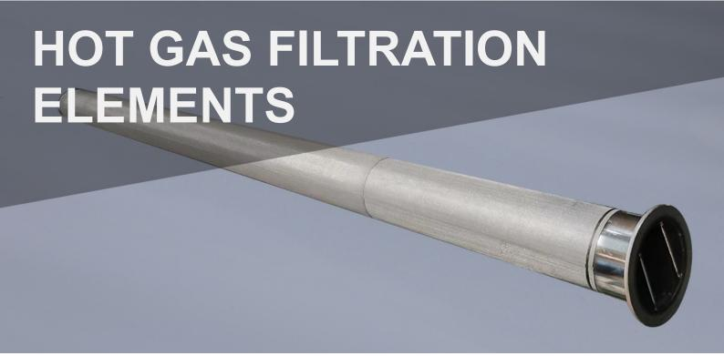
Hot gas filtration elements is one kind of sintered metal filter, with Asymmetric metal film. It's to replace the filter bags for high temperature application in bag dust collector.
