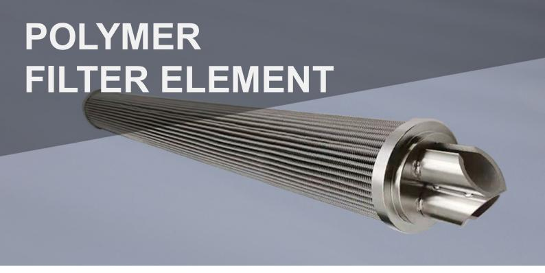
The polymer filter elements are constructed with supporting layers and filter layers that pleated together. With supporting layer, it could undertake the high pressure. With the pleated process, it increased the filtration area several times than usual candle filter. Because of this, it shorten the filter time and improve the filter effectiveness.
