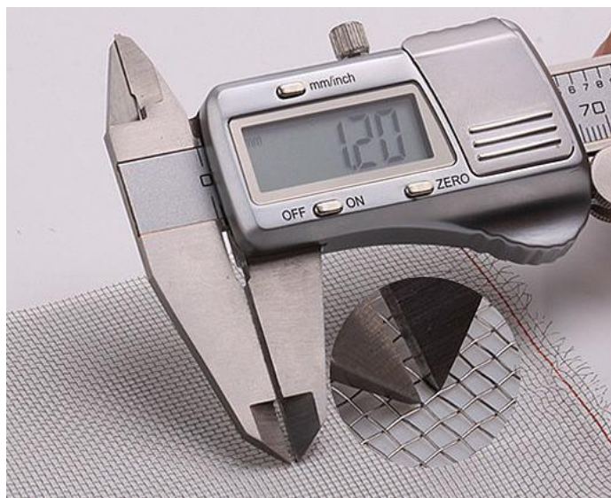
Wire Diameter Test
